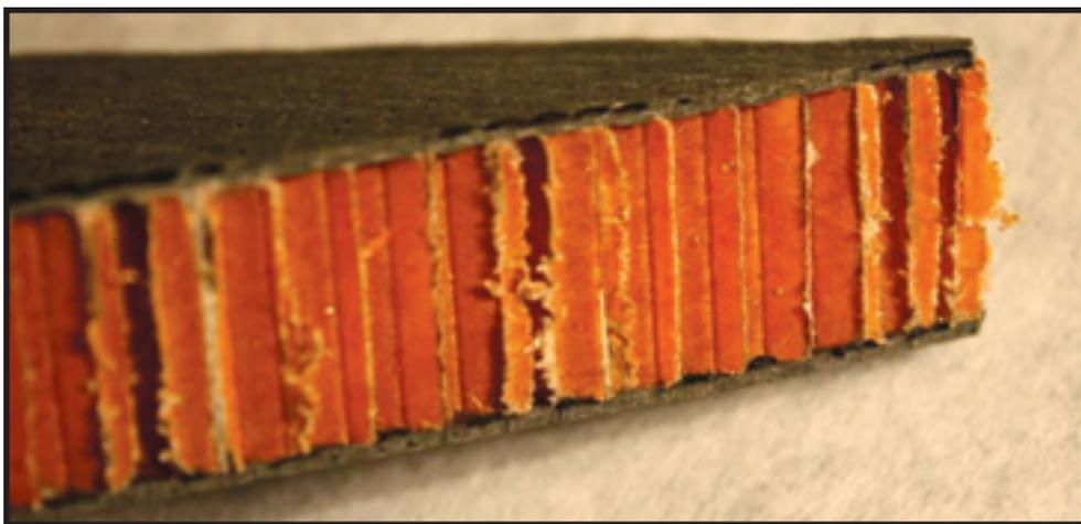
**Image 2 - Cross section of AGO's custom carbon-fiber/Nomex-honeycomb composite tube wall.**
