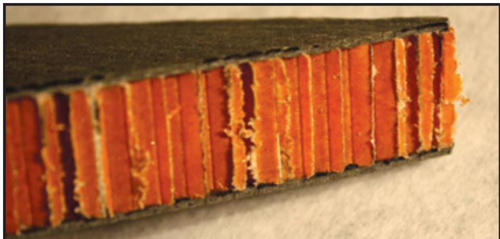
Image 2 - Cross section of AGO's custom carbon-fiber/Nomex-honeycomb composite tube wall.
