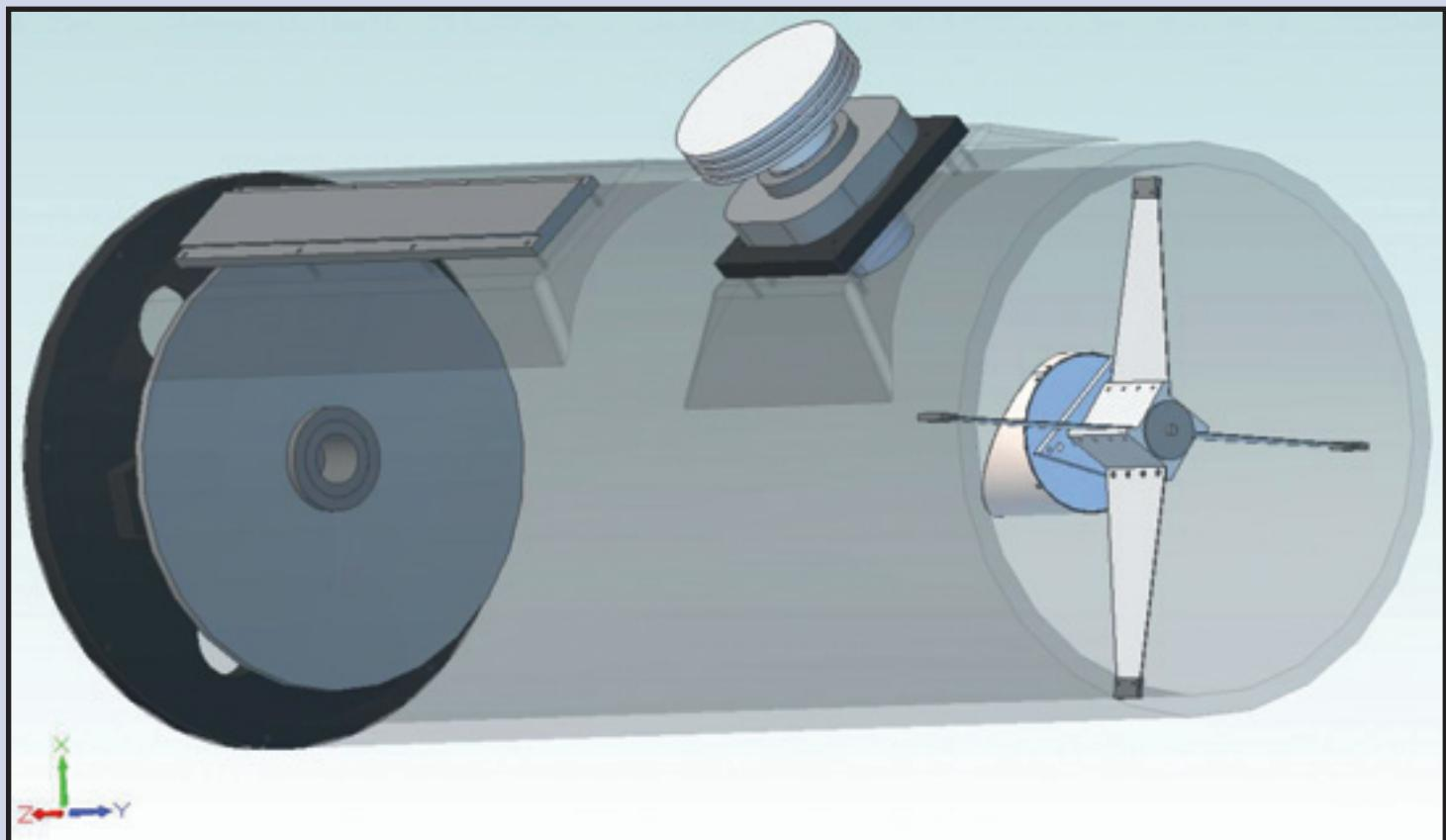
AGO Newtonian astrographs combine large aperture, fast focal ratio, and corrected optics with a lightweight, very stiff, thermally-stable carbon-fiber tube. The f/3.6 interferometrically-tested optics incorporate oversize secondaries to assure full illumination of a wide field of view. The primary and secondary mirrors feature enhanced-aluminum coatings for maximum light throughput and contrast.
