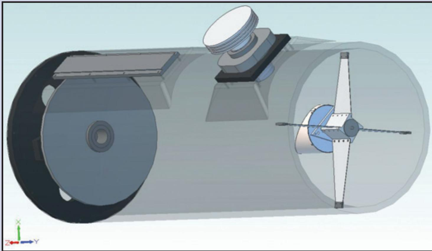
AGO Newtonian astrographs combine large aperture, fast focal ratio, and corrected optics with a lightweight, very stiff, thermally-stable carbon-fiber tube. The  $f/3.6$  interferometrically-tested optics incorporate oversized secondaries to assure full illumination of a wide field of view. The primary and secondary mirrors feature enhanced-aluminum coatings for maximum light throughput and contrast.
